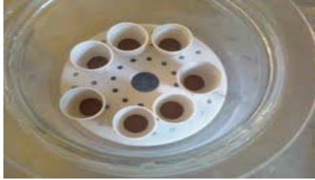
Figure 4. Soil samples cooling off [SD13] after coming out [SD14] of the muffle furnace
