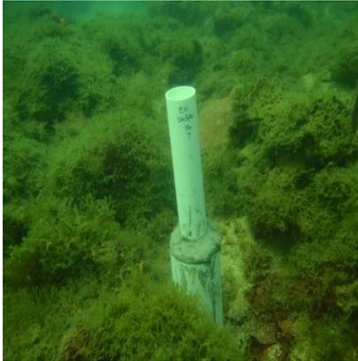
**Figure 3.** Homemade sediment trap at Ensenada 5m.
