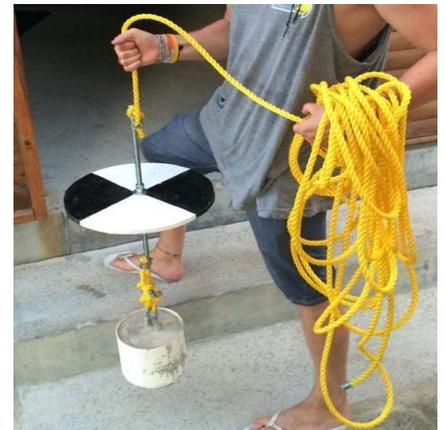
**Figure 2.** Homemade Secchi
