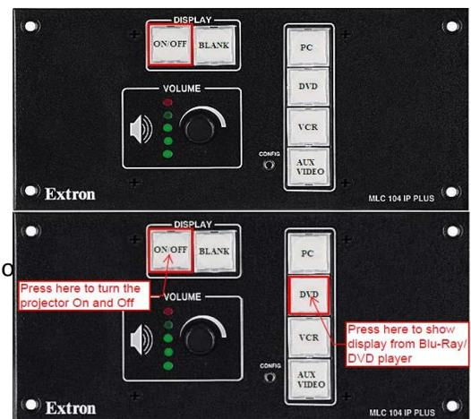
The **ON/OFF** button is flashing **AMBER** means the projector is cooling down.
